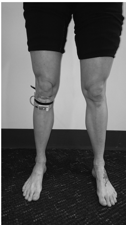
Fig. 1. Tibial acceleration position. A triaxial Noraxon DTS 3D wireless accelerometer (24 G) was attached to a steel bracket and fixed approximately 1 cm distal to the tibial tuberosity of the test limb prior to the running task.
