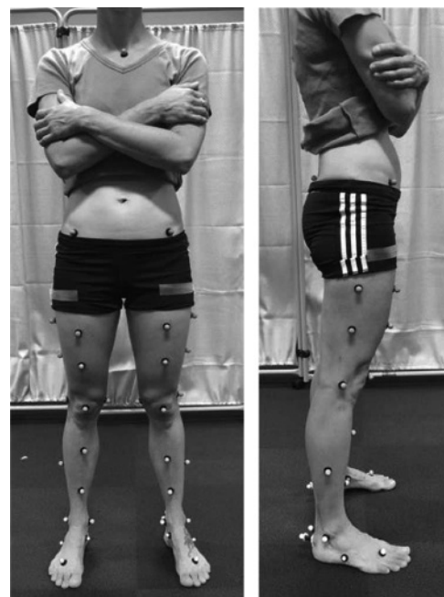
FIGURE 1 —Participant prepared for data collection. All 40 (13 mm) reflective markers were placed on the trunk, thigh, shank and foot. Participants were instructed to fold their hands across their chest (as pictured) for the static calibration.
